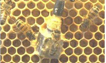
Researchers from Nottingham Trent University have developed and tested the prototype of a new device that can remotely monitor hive activity without disturbing the bees. The device picks up vibrations from the bees themselves. One common one called a "begging signal" has been used successfully to track changes in bee activity from day to night, and seasonally. The team presented their results at the 170th meeting of the Acoustical Society of America (ASA), held Nov. 2-6, in Jacksonville, Fla.
